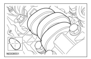
35. NOTICE: If the components are to be reinstalled, they must be installed in their original positions. Mark the components for installation into their original locations. Failure to follow these instructions may result in engine damage.
