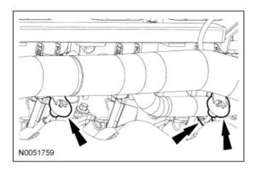
11. Disconnect the 2 engine wiring harness retainers from the LH valve cover studs.
