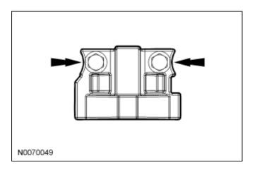
47. NOTICE: The camshaft bearing caps must be installed in their original locations. Record camshaft bearing cap locations. Record camshaft bearing cap locations. Failure to follow these instructions may result in engine damage.
