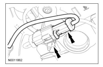
17. Disconnect the Engine Oil Pressure (EOP) switch electrical connector.
