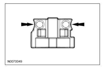
51. *NOTICE:* The camshaft bearing caps must be installed in their original locations. Record camshaft bearing cap locations. Failure to follow these instructions may result in engine damage.
