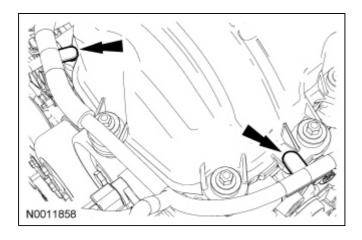
7. Remove the nut and the RH radio ignition interference capacitor.
