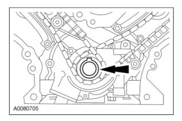
34. **NOTE:** If the camshaft lobes are not exactly positioned as shown, the crankshaft will require one full additional rotation to the 12 o'clock position.
