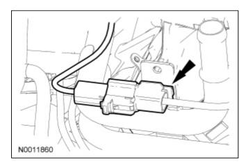
15. Disconnect the Knock Sensor (KS) electrical connector and pin-type retainer.
