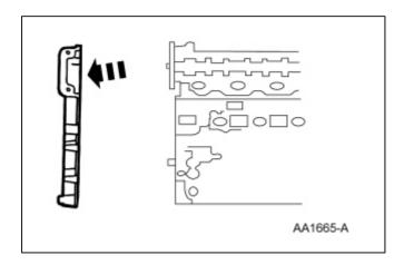
32. Remove the crankshaft sensor ring from the crankshaft.
