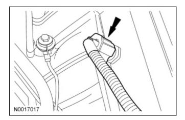
14. Detach the <u>CHT</u> sensor jumper harness electrical connector pin-type retainer.
