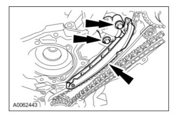
41. Remove the 2 bolts, the RH timing chain tensioner and tensioner arm.
