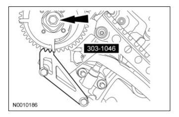
45. NOTICE: Damage to the camshaft phaser sprocket assembly will occur if mishandled or used as a lifting or leveraging device.
