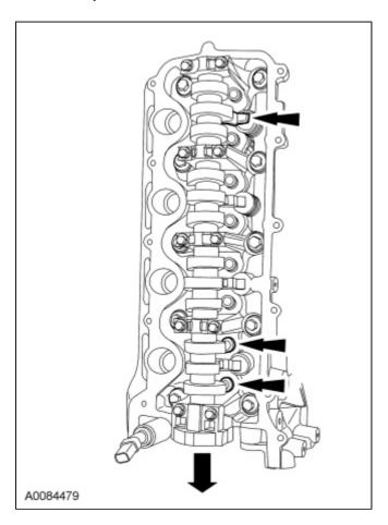
38. **NOTE:** Do not allow the valve keepers to fall off the valve or the valve may drop into the cylinder. If a valve drops into the cylinder, the cylinder head must be removed.
