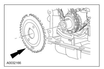
33. Position the crankshaft keyway at the 12 o'clock position.
