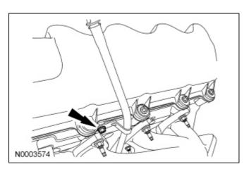
21. Remove the bolt and the RH <u>CMP</u> sensor.
