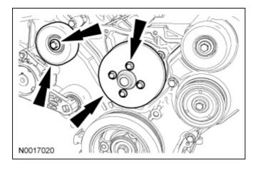
27. Remove and discard the crankshaft pulley bolt. Using the 3-Jaw Puller, remove the crankshaft pulley.
