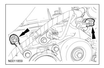
13. Disconnect the Cylinder Head Temperature (CHT) sensor electrical connector.
