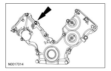
31. Remove the engine front cover from the cylinder block.
