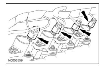
10. Disconnect the 3 engine wiring harness retainers from the RH valve cover studs.
