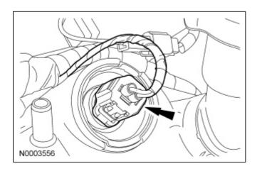
6. Detach the engine wiring harness pin-type retainers.
