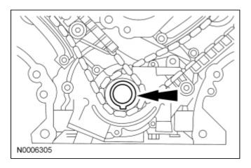
40. Remove the 2 bolts, the LH timing chain tensioner and tensioner arm.
