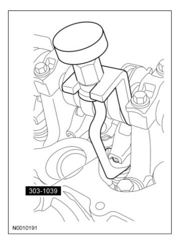
39. *NOTICE:* The crankshaft cannot be moved past the 6 o'clock position once set or engine damage may occur.
