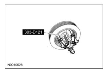
28. Using the Crankshaft Front Oil Seal Remover, remove the crankshaft seal.
