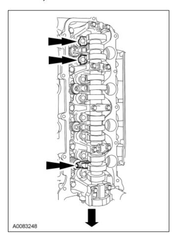
36. **NOTE:** Do not allow the valve keepers to fall off the valve or the valve may drop into the cylinder. If a valve drops into the cylinder, the cylinder head must be removed.
