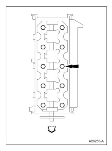
68. NOTICE: Do not use metal scrapers, wire brushes, power abrasive discs or other abrasive means to clean the sealing surfaces. These tools cause scratches and gouges that make leak paths. Use a plastic scraping tool to remove all traces of the head gasket.
