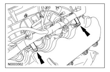
12. Detach the engine wiring harness pin-type retainers.
