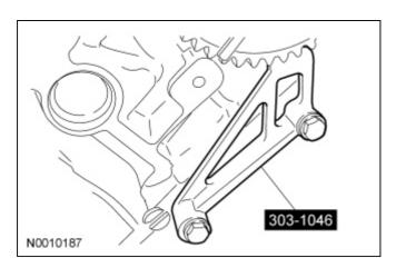
46. **NOTICE:** Remove the front thrust camshaft bearing cap straight upward from the bearing towers or the bearing cap may be damaged from side loading.
